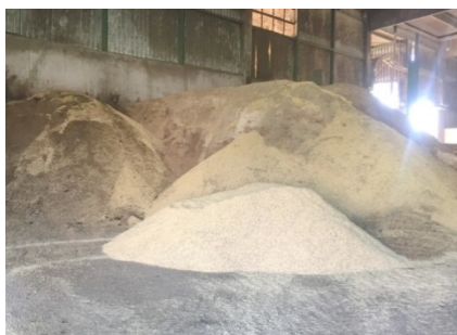
Figure 2. Biomass ashes stored in Soya Protein company rooms
