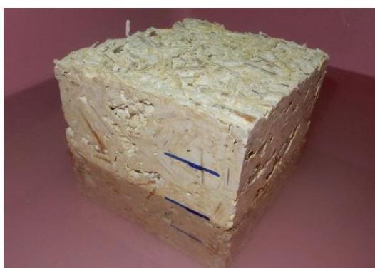
Figure 7. The water absorption of bio-concrete testing
