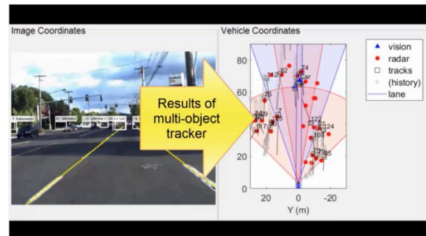
Figure 4 Results of a multi-object tracker combining radar and vision detections.
